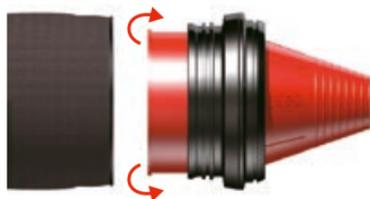
**3.** The ridge on the seal should be placed in the second groove as standard. (In some cases it can be placed in the next groove to achieve better sealing)
