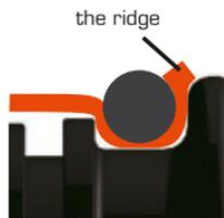
**3.** Pull the drysuit Latex seal over the Silicone seal and onto the suit ring. Check the seal is centered. Mount the o-ring into the deep groove.
