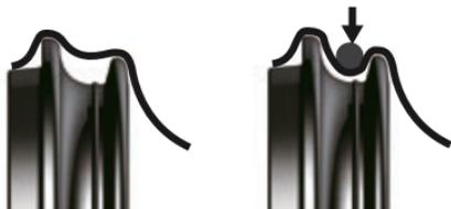
3. Fold the edge back over the o-ring and pull to adjust the overlap.
