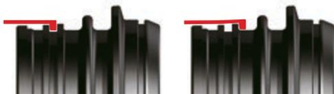
**4.** Add some waterbased lubricant on the Silicone section that slides into the suit arm. Make sure the Silicone doesn't wrinkle when pushing it into the suit.
