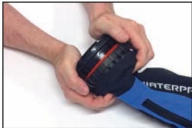
**8.** Check that the seal is properly mounted by pulling and visually inspect the inside.
